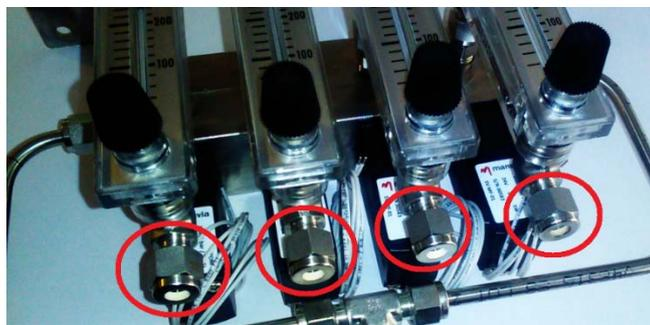
Connections are 1/8" NPTF for manifolds without rotameters:
