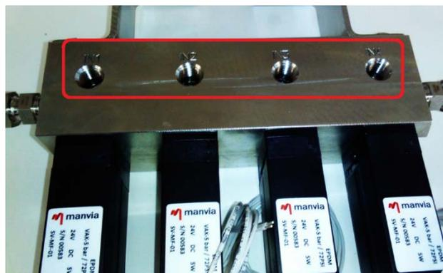
Sample outlet tubes length must be as short as possible, in order to avoid excessive response time.
