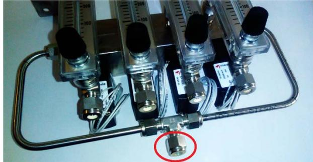
Sample outlet tubes length must be as short as possible, in order to avoid excessive response time.
